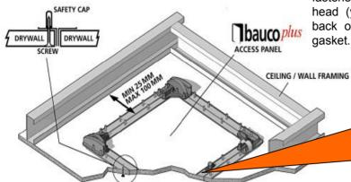
**Check contents:** Access panel, 2 installation aides (yellow), 2 retaining catches (red), 2 coil springs, fastener safety covers (red), masking disc for latch head (yellow), yellow masking cord. Fastened to back of door panel you find a self-adhesive PVC gasket.
